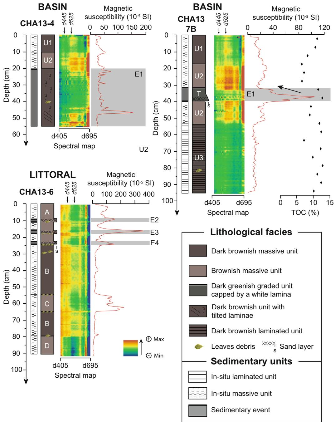
**Fig. 22.9** Multidisciplinary characterization of Lake Chauvet sediments retrieved by short gravity cores in the deep central basin (CHA13-4 and CHA13-7B) and in a littoral environment (CHA13-6). Visual descriptions of sedimentary facies are further defined (i) by sediment diffuse spectral reflectance (here plotted on a 3D diagram where the X axis represent the wavelengths, Y is the depth in core and Z the
