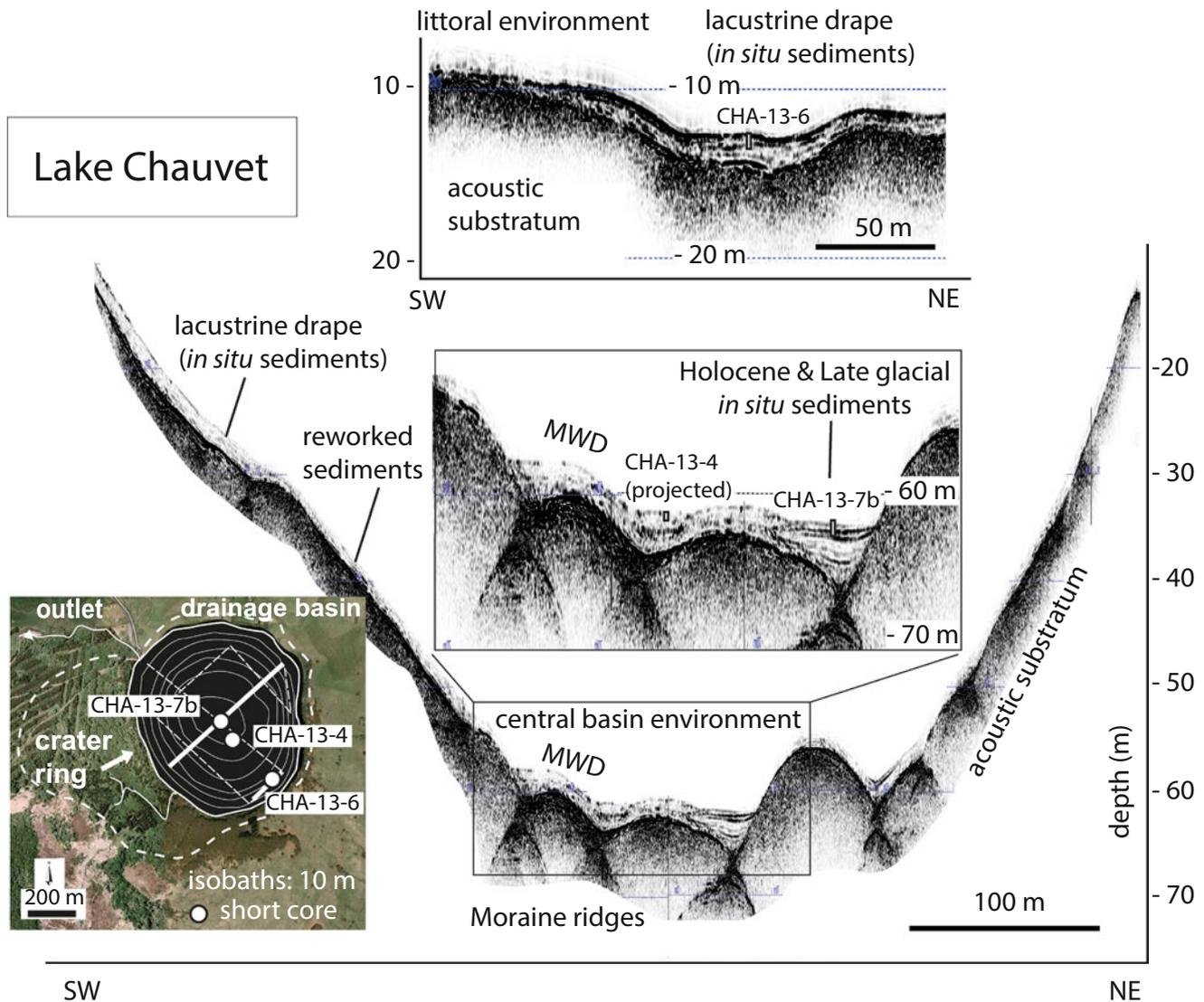
**Fig. 22.6** Lake Chauvet sub-bottom profiles (12 kHz) of a littoral environment and of the central basin. The southwestern slopes of this maar lake are unstable and a recent mass wasting deposit (MWD) can be identified within the deep central basin where moraine ridges are ponded by Late glacial and Holocene lacustrine sediments. The bathymetric
