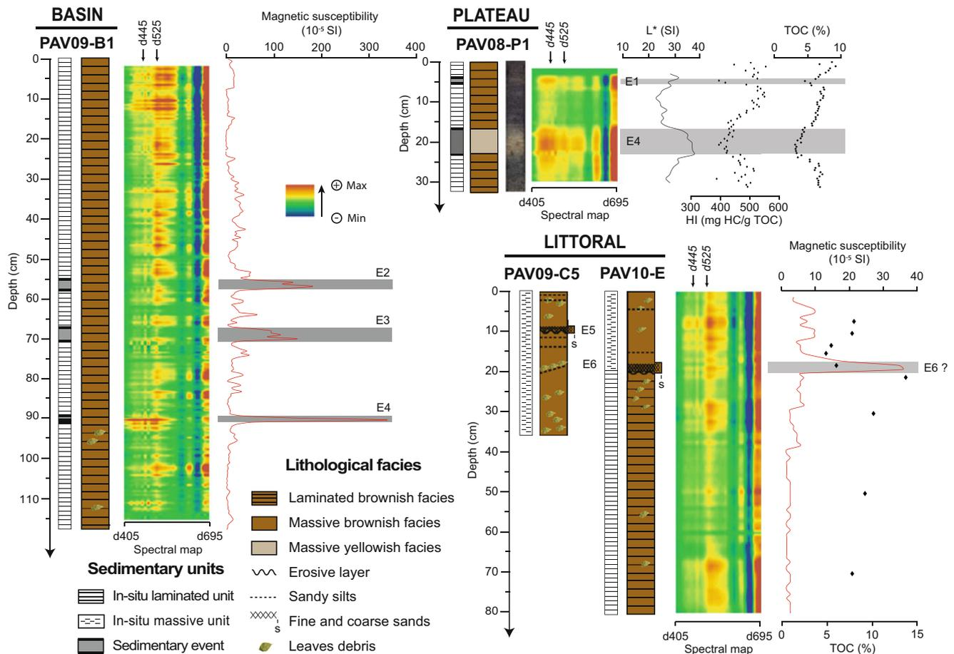
**Fig. 22.8** Multidisciplinary characterization of Lake Pavin sediments retrieved by short gravity cores, in the deep central basin (PAV09-B1), on the plateau (PAV8-P1) and in littoral environments (PAV09-C5 and PAV10-E). Visual descriptions of sedimentary facies are further defined (i) by sediment diffuse spectral reflectance (here plotted on a 3D diagram where the X axis represent the wavelengths, Y is the depth in core and Z the first derivative value for the corresponding wavelength (in
