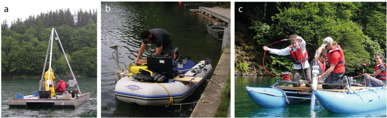
**Fig. 22.3** Recently available geological data from in Lake Pavin and Lake Chauvet discussed in this chapter include short gravity coring performed from an UWITEC platform in 2008 (a); high resolution seismic
